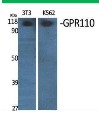
Western Blot analysis of various cells using GPR110 Monoclonal Antibody
