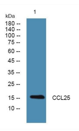
Western Blot analysis of various cells using CCL25 Monoclonal Antibody
