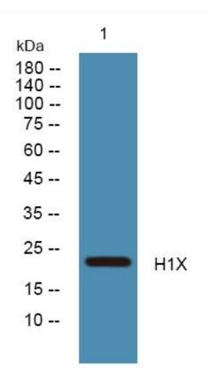
Western Blot analysis of various cells using H1X Monoclonal Antibody
